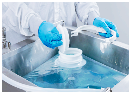
3" OR 4" PORT FOR POWDER ADDITION
