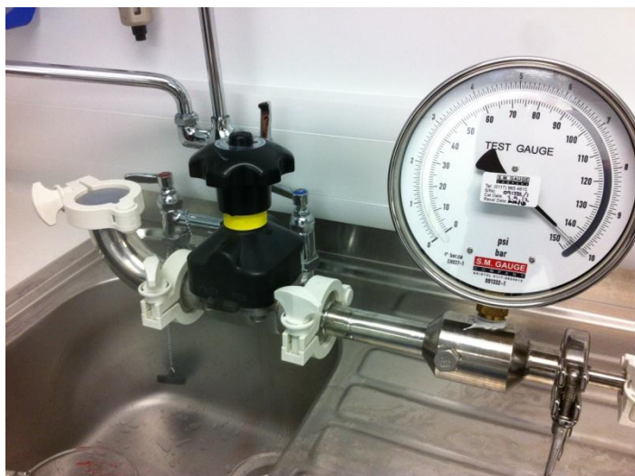
Photos showing clamped 1 - ½" End Cap, Test Pressure, and Wing Nut Torque value.
