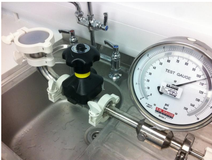
Photos showing clamped 2 ½" End Cap, Test Pressure, and Wing Nut Torque value.
