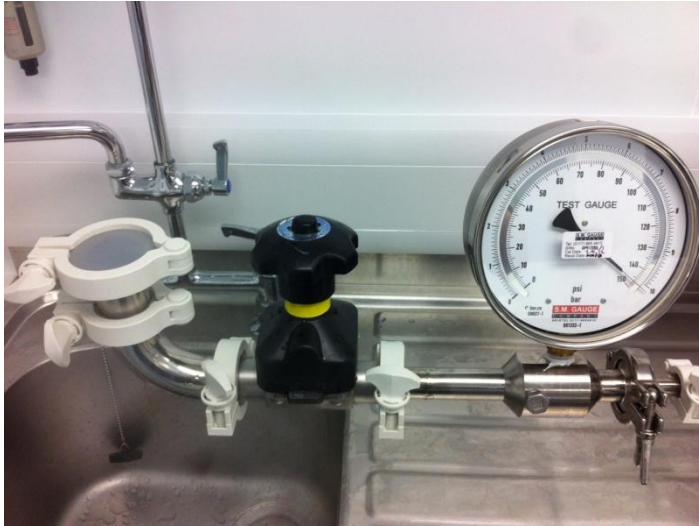
Photos showing clamped 2" End Cap, Test Pressure, and Wing Nut Torque value.
