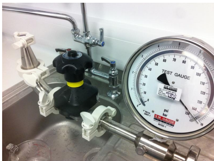
Photos showing clamped ¾" End Cap, Test Pressure, and Wing Nut Torque value.
