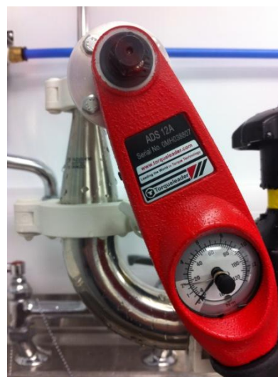
Photos showing clamped ¾" End Cap, Test Pressure, and Wing Nut Torque value.
