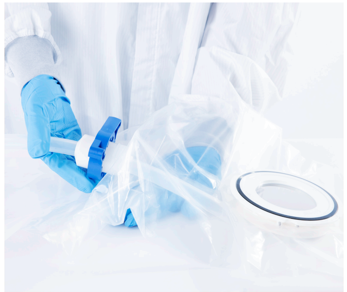
THRU TC CONNECTED TO A BETA BAG FOR ISOLATOR TRANSFER
