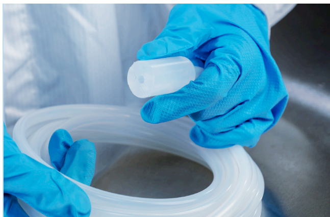
SINKER FOR FLUID ADDITION AND REMOVAL IN A BOTTLE/CARBOY
